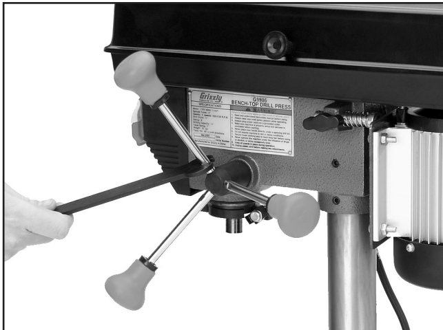
Figure 8. Tightening the downfeed handles.
